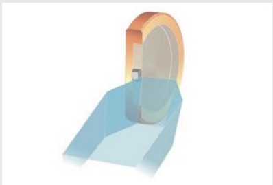
Cryo trimming tissue HP frozen in a flat specimen carrier
